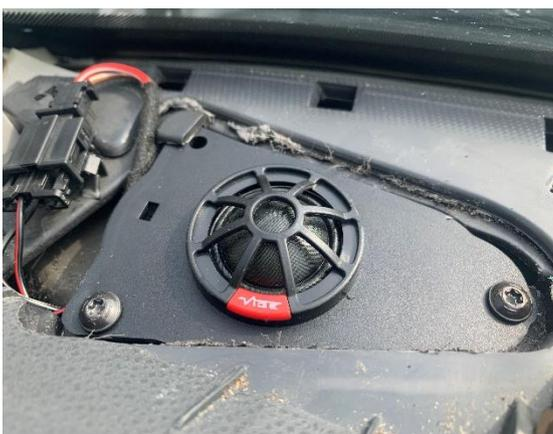
22. Reconnect the tweeter in the vehicle and secure the tweeter mount using the T15 screw previously removed. Test for correct operation and refit the dash cover
