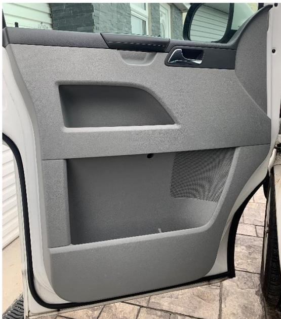
1. To access the door speaker, first carefully remove the door card. This is secured with 6 x T25 Torx screws and plastic panel clips. Ensure all screws and clips are correctly removed and retained for re-installation
