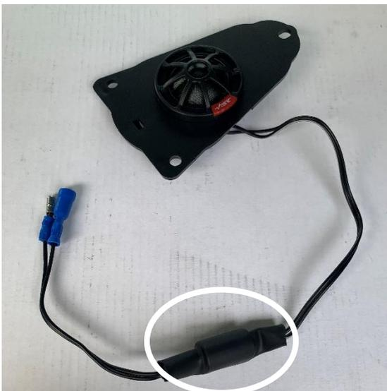
21. Cut back the tweeter wiring ensuring the crossover/capacitor remains in-line with the positive wire (Black/White). Add the blue bullet connectors provided and connect to the tweeter connector. Ensure the Polarity is correct and connected as below
