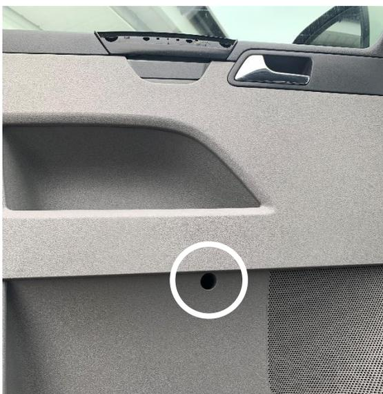
4. Remove the single T25 Torx screw located in the centre of the door card
