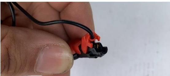
18. For vehicles that are not fitted with factory tweeters in the dash, the OPTI1C tweeter wires will need to be routed to behind the stereo. Connect the T Crimp connectors as shown to the Tweeter wires and clamp closed using pliers or similar.
