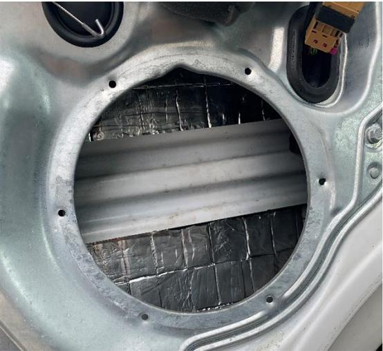
16. Ensure the door panel is clean and free from grease and dirt. Apply the self-adhesive sound deadening to the door panel directly behind the speaker as shown. For maximum coverage cut the sound deadening in half and place above and below the door strengthening bar
