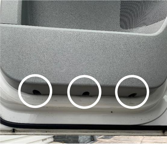
5. Remove the three T25 Torx screws located along the bottom edge of the door card. Once removed, use a trim removal tool to carefully release the plastic clips securing the door card to the door
