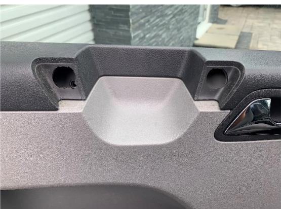
3. With the Torx screws removed, remove the handle completely from the door card.
