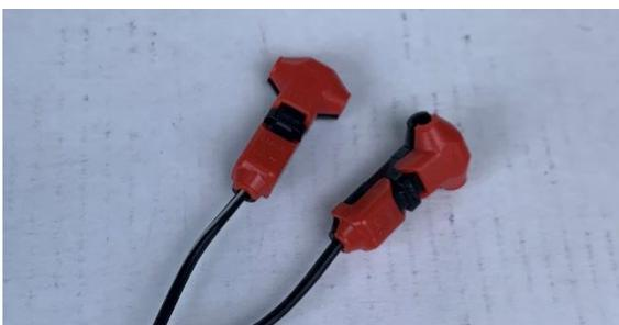
**Please make sure the included crossover is used. This can vary from the kit order from inline to separate yellow cap. This should be used on the positive cable**
