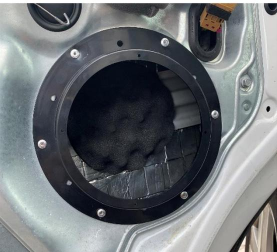
10. Fix the speaker bracket to the door panel by lining up the securing holes and using nuts & bolts or screw/rivets **(not provided)** to secure the mounting bracket to the door
