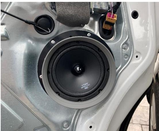
14. Connect the speaker spade terminals to the woofer ensuring the polarity is correct (Red Positive +, Black Negative -) Line up the holes and silicone baffle and use the screws provided to secure to the speaker adaptor
