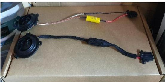
17B. The tweeters are to be fitted into the original place and plug into the original position.
