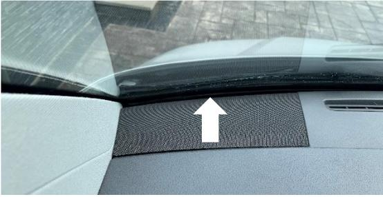
15. To remove the factory tweeter (if fitted) first use a trim removal tool to remove the dash cover. Lift the front edge first and remove completely
