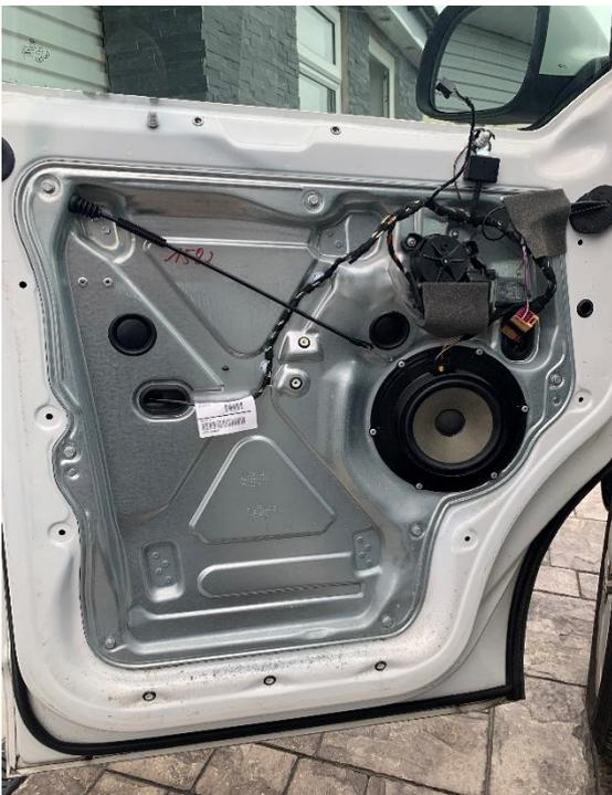
7. Once the door card is removed fully, store safely to avoid damage.
