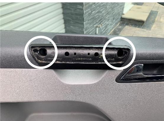
2. Using a trim removal tool, remove the plastic trim from the centre of the door handle then remove the two T25 Torx screws located behind. (We recommend using the VIBE CLTRT-V7 trim removal tools available from any VIBE authorised dealer)
