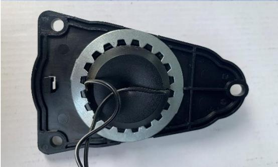
Secure the OPTI1C tweeter to the new tweeter mount using the metal locking ring provided.
