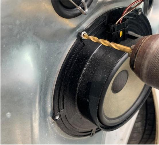
15. The factory speaker is secured to the door using rivets. To remove the speaker, drill out the rivets using a 5mm drill bit. Take care not to damage the vehicle and ensure protective eyewear is worn. Once all rivets are removed, unplug the speaker, and remove.
