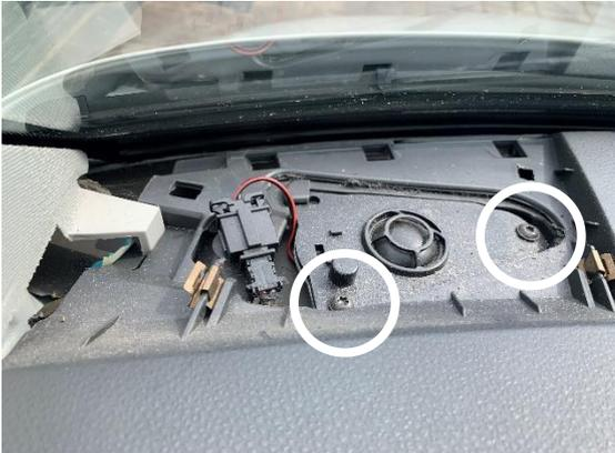
16. Remove the tweeter (if fitted) by removing the two T15 Torx screws securing the tweeter mount to the dash and unplugging the tweeter connector. Safely retain the mounting screws for reinstallation
