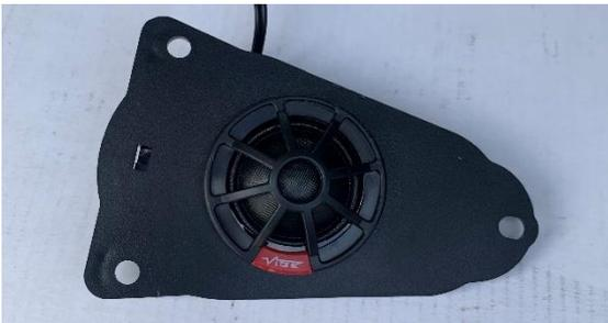
17. Before fitting the new tweeters, please make sure the crossover or capacitor is used to protect the tweeter. (See Section 21 for details.)
