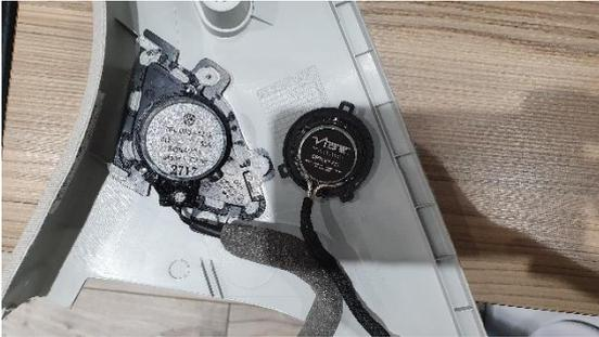
16B. Once removed the Tweeter is now able to be removed. These are plastic welded into place from factory and can easily be removed with the use of heat and a small amount of pressure.
