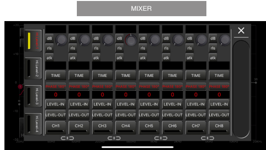
Mixer allows any input channel to be mapped to any output channel. Especially useful when you need the full 10 channel output from a stereo source such as a phone.
