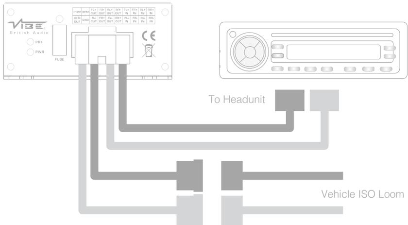
**NOTE :** If your vehicle does not have a standard ISO connector (for example a quadlock connector) it will be necessary to purchase a separate vehicle specific T-Harness connector
