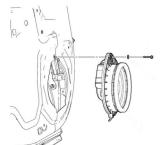
• Attach the vehicle specific adaptor ring to the door / door card.
