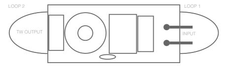
No loop cut: 0dB Cut loop 1: -2.5dB Cut loop 2: -3.5dB
